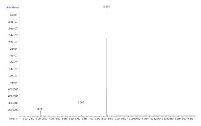
Additional peaks present in chromatogram: internal standards (3.217 min and 6.287 min)
