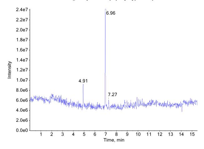
Additional peaks present in chromatogram: internal standards (4.91 min and 7.27 min)
