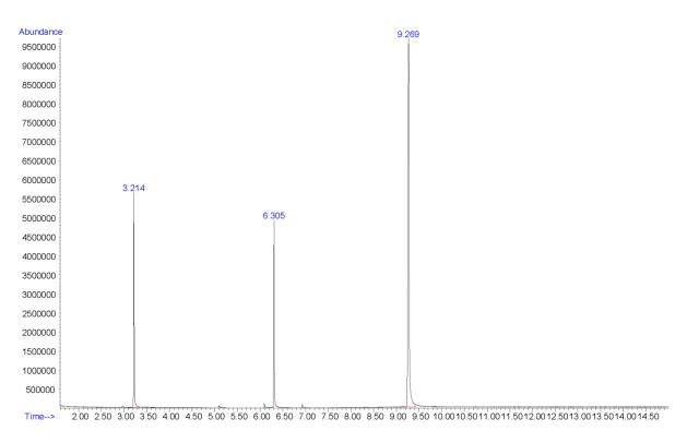
Additional peaks present in chromatogram: internal standards (3.214 min and 6.305 min)
