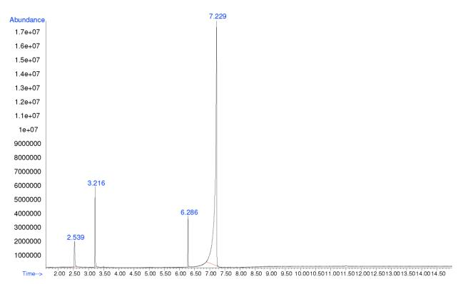
Additional peaks present in chromatogram: not a controlled substance (2.539 min), internal standard 1 (3.216), internal standard 2 (6.286)
