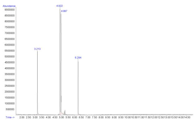
Additional peaks present in chromatogram: internal standard (3.213 min), not a controlled substance (4.922 min), and internal standard (6.294 min)
