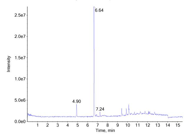
Additional peak present in chromatogram: internal standards (4.90 min and 7.24 min)
