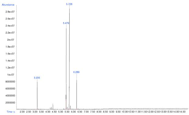
Additional peaks present in chromatogram: internal standard 1 (3.205 min), N-ethyl pentylone (5.479 min), and internal standard 2 (6.289 min)
