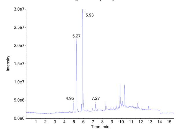
Additional peaks present in chromatogram: internal standard 1 (4.95 min), N-ethyl pentylone (5.27 min), and internal standard 2 (7.27 min)
