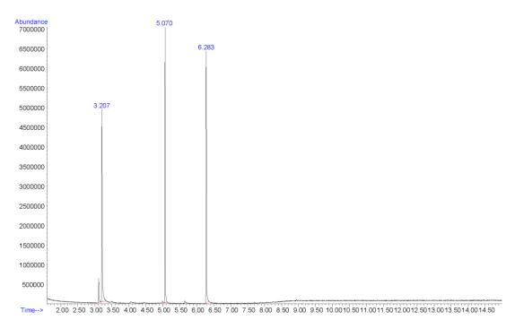
Additional peaks present in chromatogram: internal standards (3.207 min and 6.283 min)
