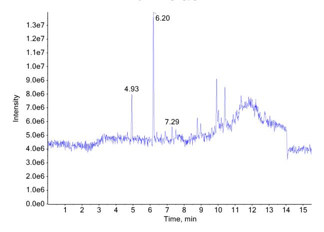
Additional peaks present in chromatogram: internal standards (4.93 min and 7.29 min)
