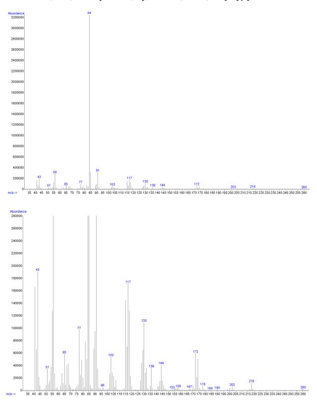
EI (70 eV) Mass Spectrum (Top) and 10x (Bottom): Isopropylphenidate
