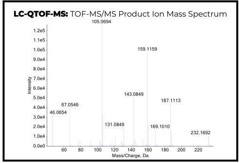
**Confirmation Using Drug Standard:** Reference material for deoxymethoxetamine (Batch: 0619632-3) was purchased from Cayman Chemical (Ann Arbor, MI, USA). The analyte was confirmed to be deoxymethoxetamine based on retention time (sample: 5.18 min vs. standard: 5.27 min) and mass spectral data comparisons.
