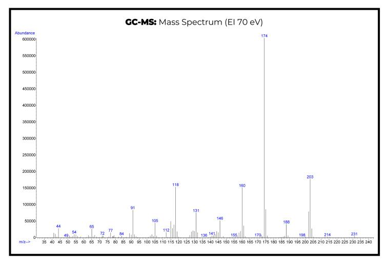
**Confirmation Using Drug Standard:** Reference material for deoxymethoxetamine (Batch: 0619632-3) was purchased from Cayman Chemical (Ann Arbor, MI, USA). The analyte was confirmed to be deoxymethoxetamine based on retention time (sample: 4.87 min vs. standard: 4.84 min) and mass spectral data comparisons.
