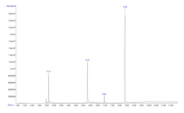
Additional peaks in chromatogram: internal standards (3.12 and 5.79 mins), unknown brominated analyte (6.94 min)
