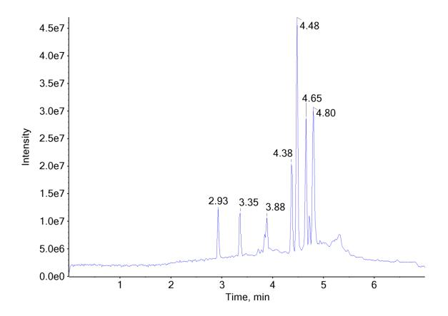
Additional peaks present in chromatogram: internal standard 1 (2.93 min), not a controlled substance (3.35 min), internal standard 2 (3.88 min), not a controlled substance (4.48 min), MMB-FUBINACA [FUB-AMB] (4.65 min), not a controlled substance (4.80 min)
