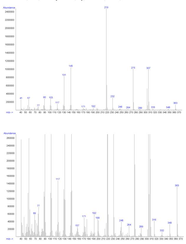
EI (70 eV) Mass Spectrum (Top) and 10x (Bottom): 4F-MDMB-BINACA
