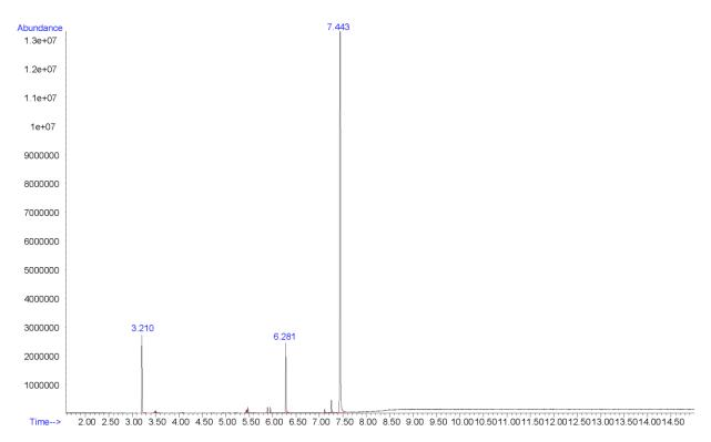
Additional peaks present in chromatogram: internal standard 1 (3.210 min) and internal standard 2 (6.281 min)
