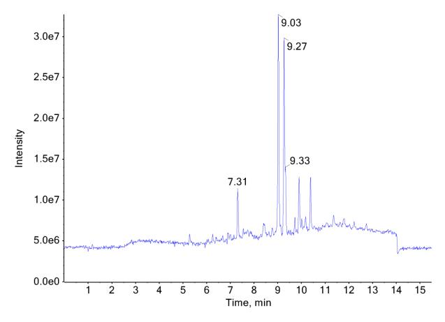
Additional peaks present in chromatogram: internal standard (7.31 min), 5F-EMB-PICA (9.27 min), and 5F-MDMB-PICA (9.33 min)
