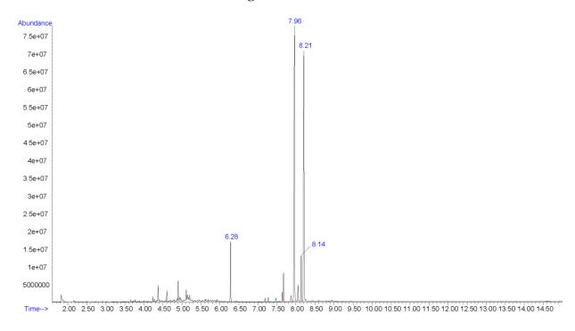
Additional peaks present in chromatogram: internal standard (6.28 min), 5F-MDMB-PICA (8.14 min), and 5F-EMB-PICA (8.21 min)
