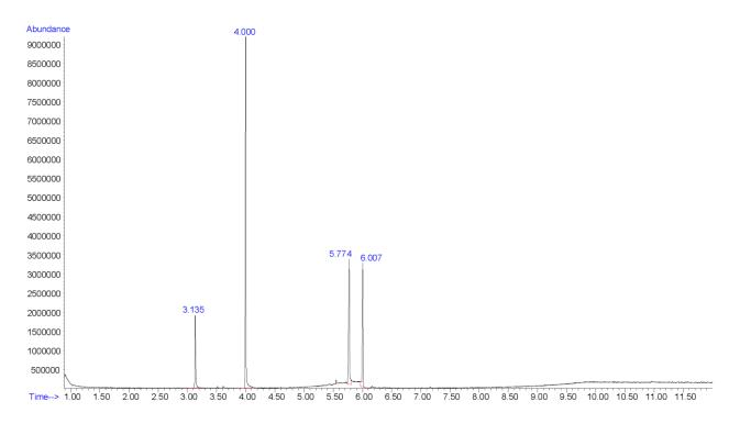
Additional peaks present in chromatogram: internal standards (3.135 min), breakdown product (4.000), internal standard (6.282 min)
