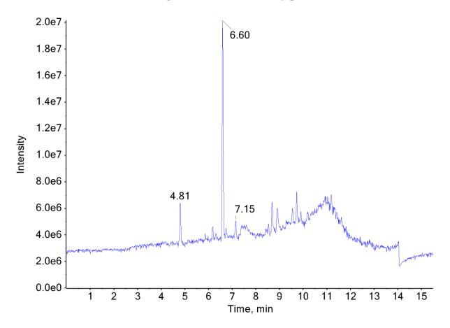
Additional peaks present in chromatogram: internal standards (4.81 min and 7.15 min)
