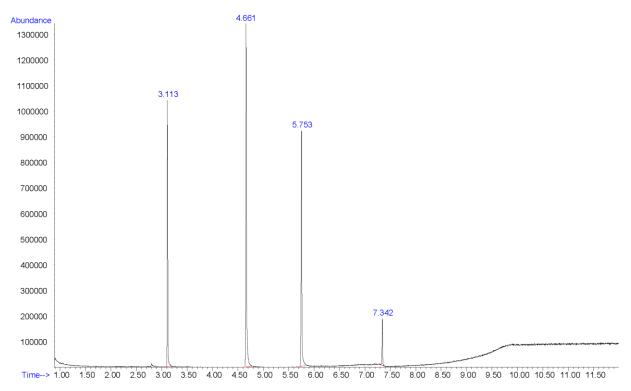
Additional peaks present in chromatogram: internal standard (3.113 min), 2C-C [thermal degradation product] (4.661 min), internal standard (5.753 min), 25C-NBOH suspected formyl artifact (approx. 7.342)
