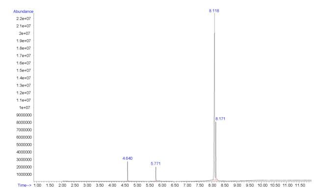
Additional peaks present in chromatogram: internal standard monoacetyl- derivative (4.640 min), internal standard (5.771 min), 25C-NBOH monoacetyl- derivative (8.118 min), 25C-NBOH diacetyl- derivative (8.171 min)
