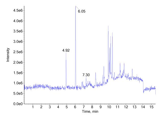
Additional peaks present in chromatogram: internal standards (4.92 min and 7.30 min)
