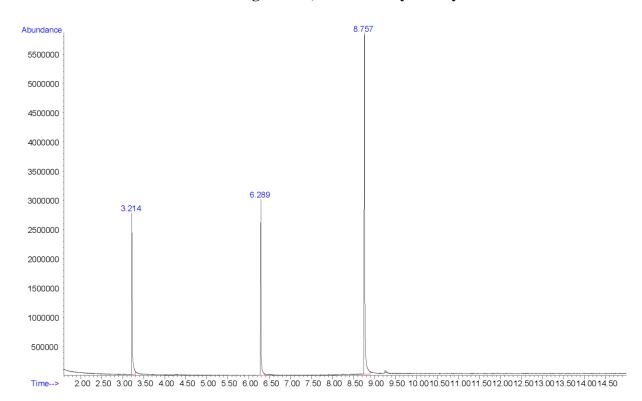
Additional peaks present in chromatogram: internal standards (3.214 min and 6.289 min)
