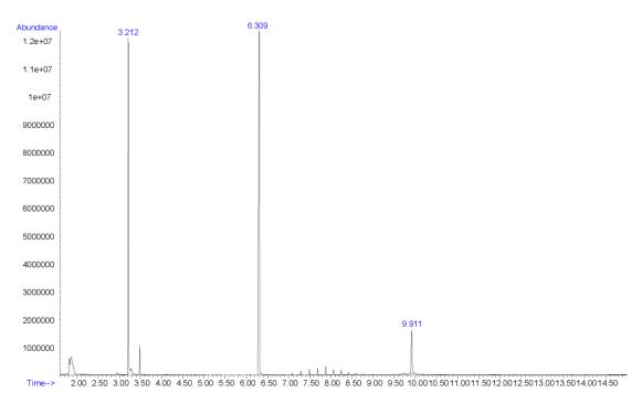
Additional peaks present in chromatogram: internal standards (3.212 min and 6.309 min)
