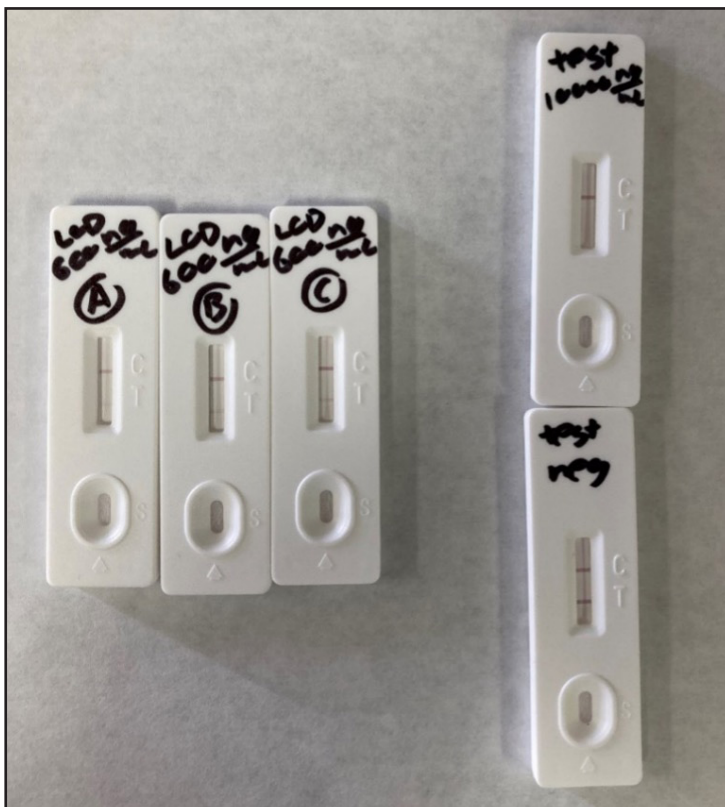
Figure 1-2: Concentration Below Limit of Detection (Left: 600 ng/mL of xylazine standard in triplicate; Top right: Positive control at 100,000 ng/mL; Bottom right: Negative control)
