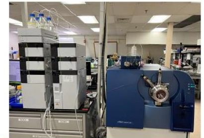
Sciex TripleTOF® 5600+ LC-TOF-MS
