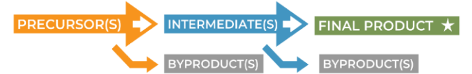
Figure 4: Generic flow of chemicals during drug synthesis. Illustration shows when byproducts may be formed during the synthesis process.
